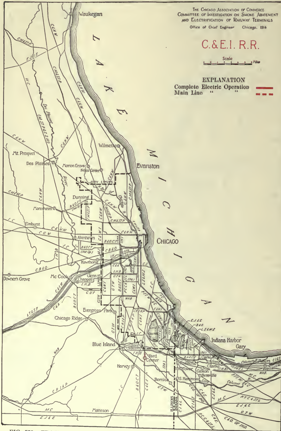
FIG. 550. TRACKAGE TO BE ELECTRIFIED BY THE CHICAGO & EASTERN ILLINOIS RAILROAD
